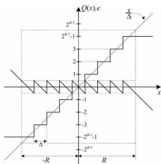
Figure 12: Uniform scalar mid-thread quantizer
